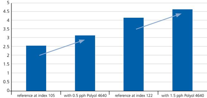
Hardness improvement in 20 kg/m<sup>3</sup> density TDI flexible foam with addition of 0.5 to 1.5 parts of Polyol 4640
